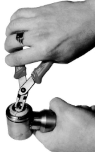
4. Check the condition of the Electrode Assembly. If it is to be removed, grip the Electrode Assembly with the special Electrode Pliers provided, and pull firmly out from the torch body. (See illustration right).
